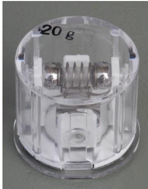
fig 3: Indicator not tripped
