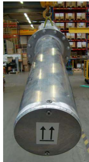
Figure 4: oil tank (long term storage)
