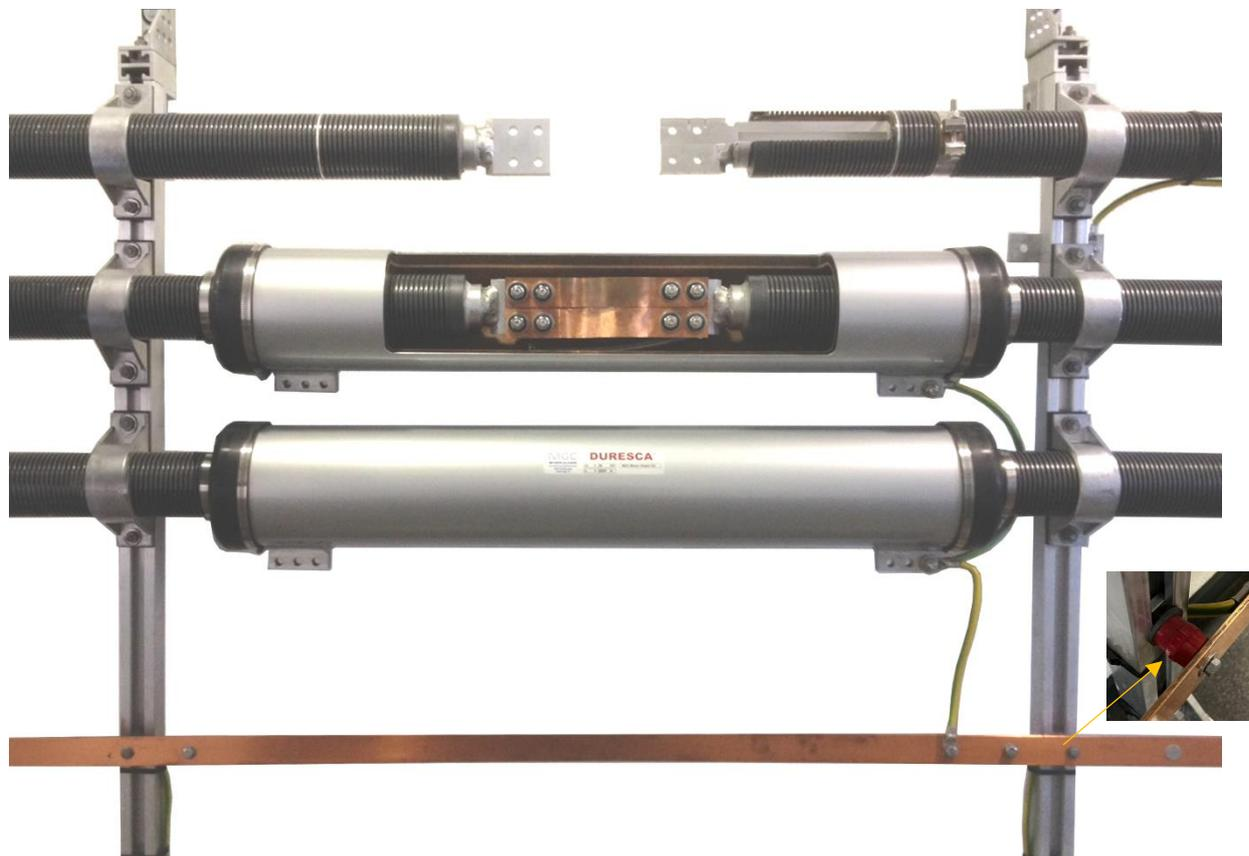
Figure 7: Display model with cut busbars and sleeves
