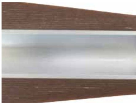
Cut from an RIP active part
