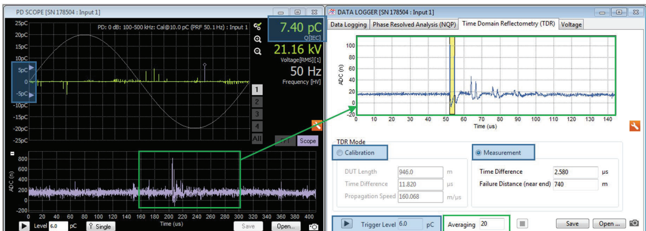
Fig. 3: PD detector cable site location with PD level triggering and signal averaging.
