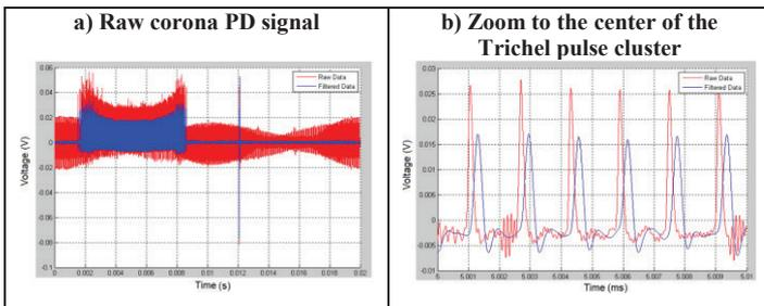
Fig. 9: Oscilloscope measurements (2 MHz low-pass filter)
