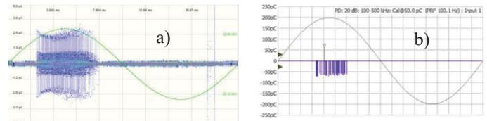
Fig. 3: Pulse polarity: a) ambiguous recognition due to fixed dead time, b) distinct recognition without ambiguity.
