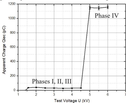
Fig. 2: Charge-voltage dependence of corona discharge
