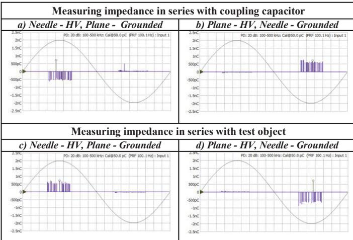
Fig. 5: Influence of the measuring impedance and HV source location – Pre-breakdown streamers – Phase IV
