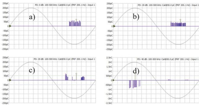
Fig. 1: Corona development phases in the pulse ( $\Phi$ -q) diagram: a) Phase I, b) Phase II, c) Phase III, d) Phase IV.
