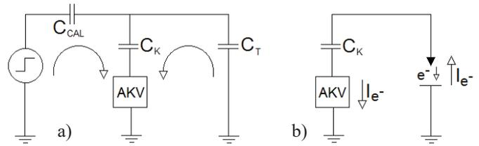
Fig. 6: Influence of the measuring circuit to the pulse polarity.
