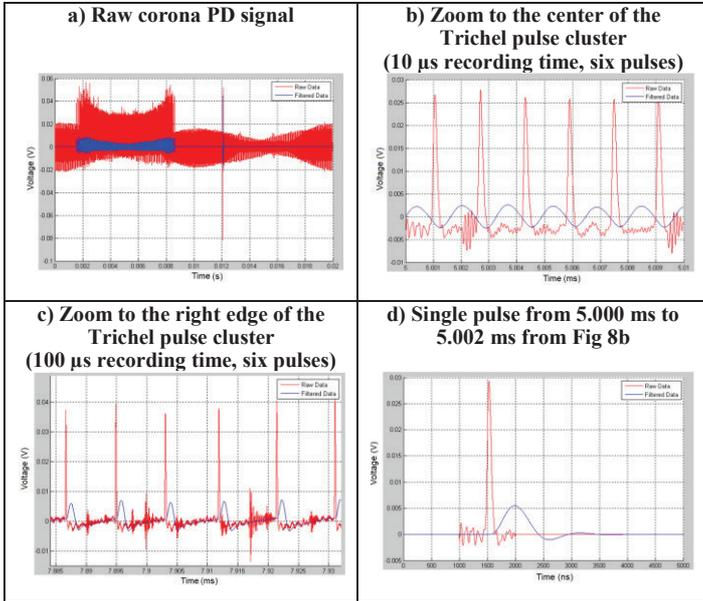
Fig. 8: Oscilloscope measurements (0.5 MHz low-pass filter)
