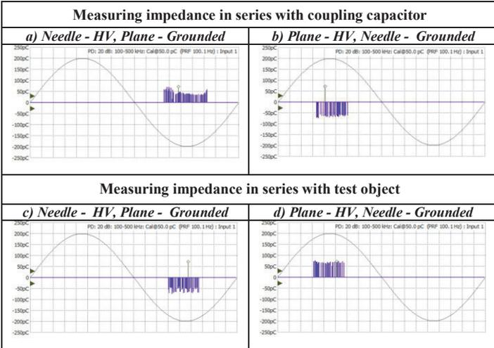
Fig. 4: Influence of the measuring impedance and HV source location – Trichel pulses – Phases I – III
