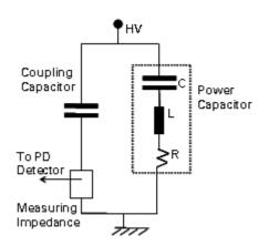
Fig 1. Classical PD Measurement Circuit
