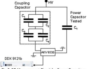
Fig 2. PD Measurement Circuit for Power Capacitors
