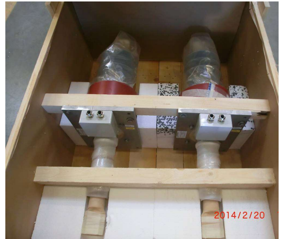
Figure 2: bushing with CT
